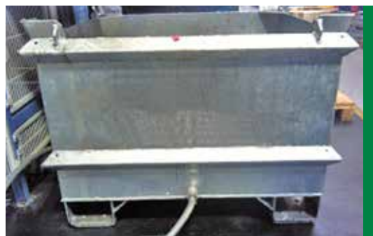
4 COLLECTION CONTAINER WITH DOUBLE-WALLED BASE, SWARF FILTER AND DISCHARGE DEVICE FOR EMULSIONS
