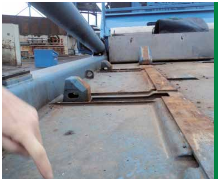
10 TIPPING CONTAINER VEHICLE WITH THROUGH-WELDED FLOOR PLATE AND CHAMFERING FOR LEAKPROOF TRANSPORTATION OF SWARF
